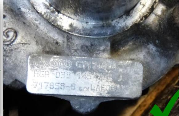
The type plate of the core must not be removed. Turbo chargers without or with a manipulated type plate cannot be accepted, as an unequivocal identification for the return to the manufacturer is no more possible.
