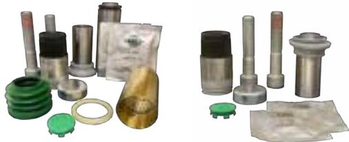
Guide Sleeve and Tappet Boot Kits To Fit All 5C1450 / 5C1455 Calipers
