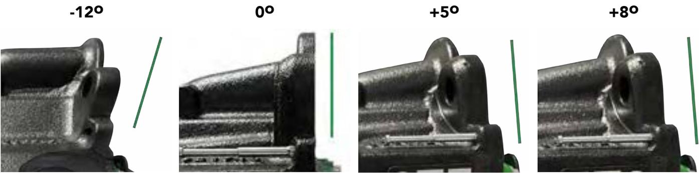
For radial calipers (LNR225) the mounting angle ranges from  $+86^{\circ}$  to  $+93^{\circ}$ .
