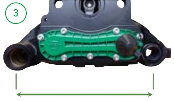
If there are no bolts visible it is an LB225, LV225 or LNR225 brake. The mounting angle of the LNR brake (see earlier) makes it easy to identify. To distinguish between the LB225 and the LV225:
