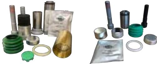
Guide Sleeve and Tappet Boot Kits To Fit All 5C6900 / 5C6905 Calipers
