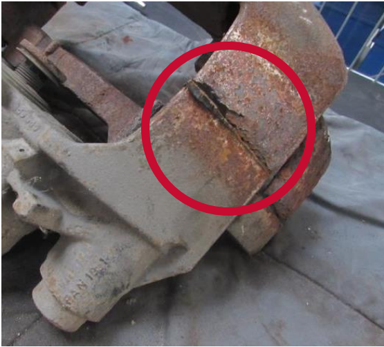
Cracked frame or carrier
